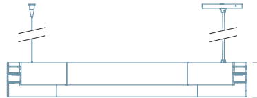
RPD06 E1 Section A-A Cut View: The R1 has longer exterior length rings.
