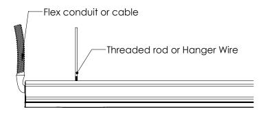
SUPPORT TO STRUCTURE MUST BE PROVIDED VIA BLOCKING, HANGING WIRE OR THREADED **ROD (ALL BY OTHERS)**
